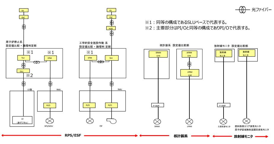
TLU: Trip Logic Unit DTM: Digital Trip Module OLU: Output Logic Unit LD: Load Driver
