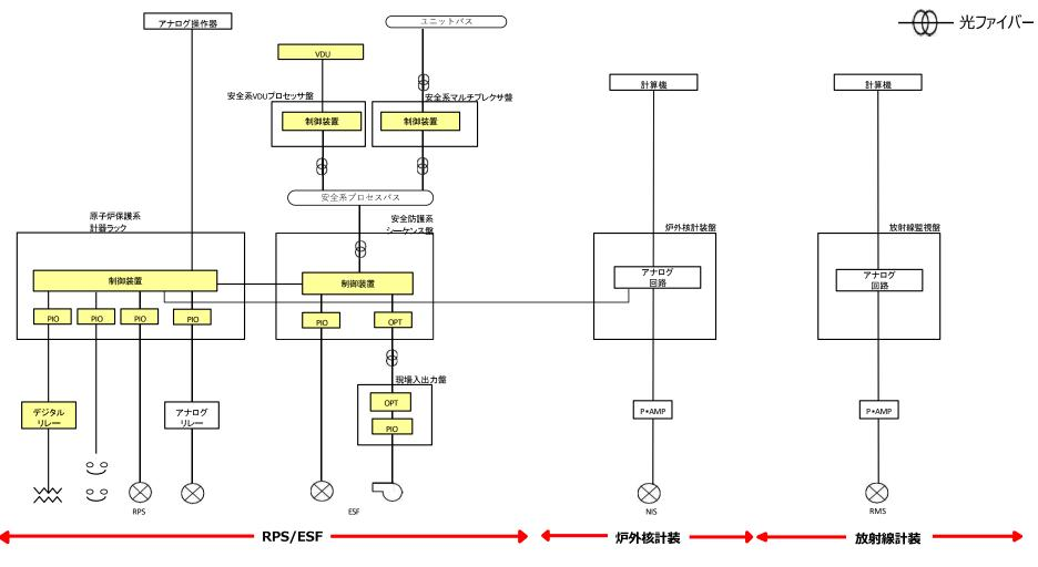
RPS: Reactor Protection System ESF: Engineered Safety Features VDU: Visual Display Unit PIO: Process Input Output
